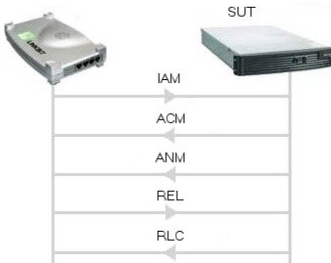
ISUP call flow used for CPS measurements.
