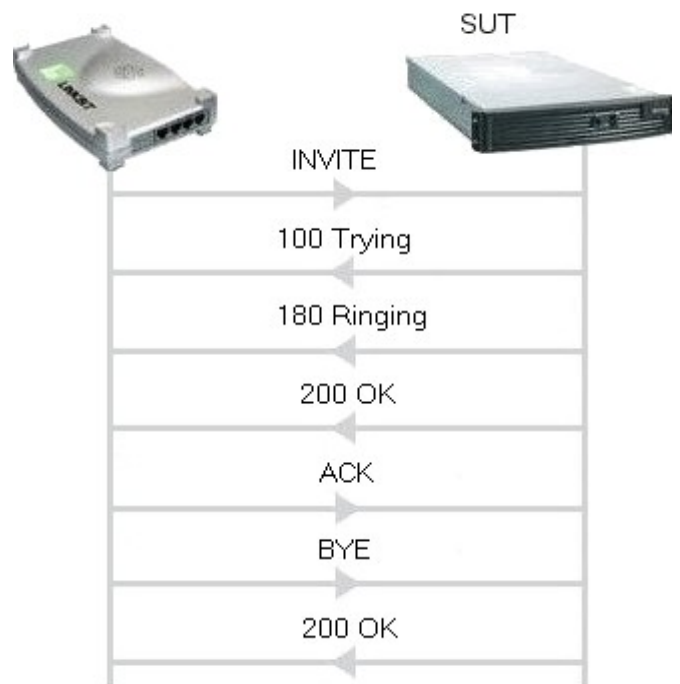
SIP call flow used for CPS measurements.
